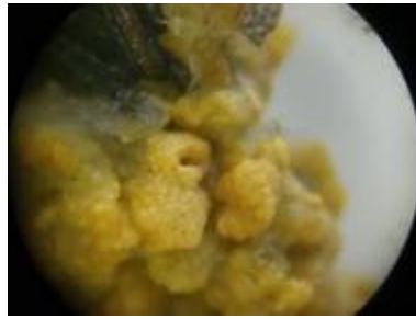
Figure 9: Microscope picture of precipitation of metal sulphide (1:500)
