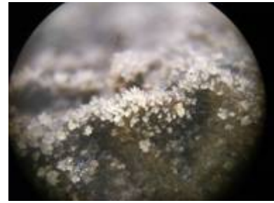
Figure 10: Microscope picture of precipitation of salt (1:500)
